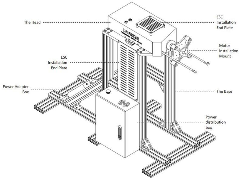
FIG 4-2-1 Thrust stand structure
