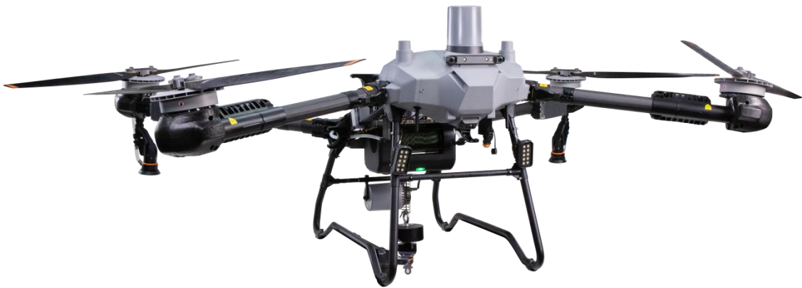
FIG 3-1-1 UAV platform equipped with XD-55 UAV payload winch system
