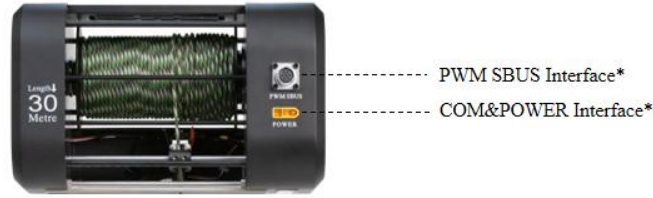
FIG 3-2-3 Diagram of XD-55 line interface
