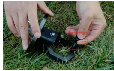
FIG 7-1-2 Pull out the pin
