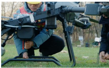
FIG 7-1-1 Lower the cable to a sufficient length
