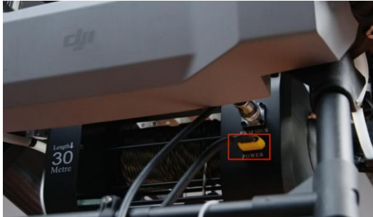
FIG 5-2-2 Insert the cord into the winch power port
