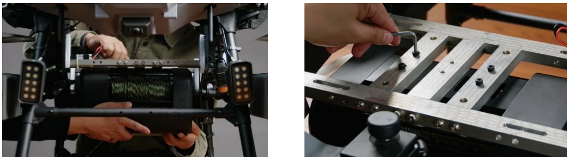
FIG 5-1-1 The installation of the winch body on the aircraft platform
