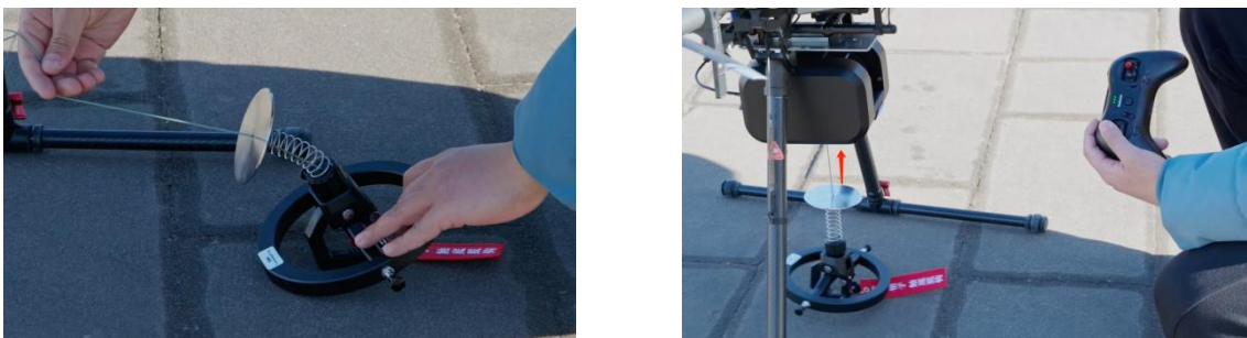
FIG 5-4-3 Ensure that the rope is not tangled & the unhooker is reset
