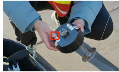
FIG 7-2-2 open the hook
