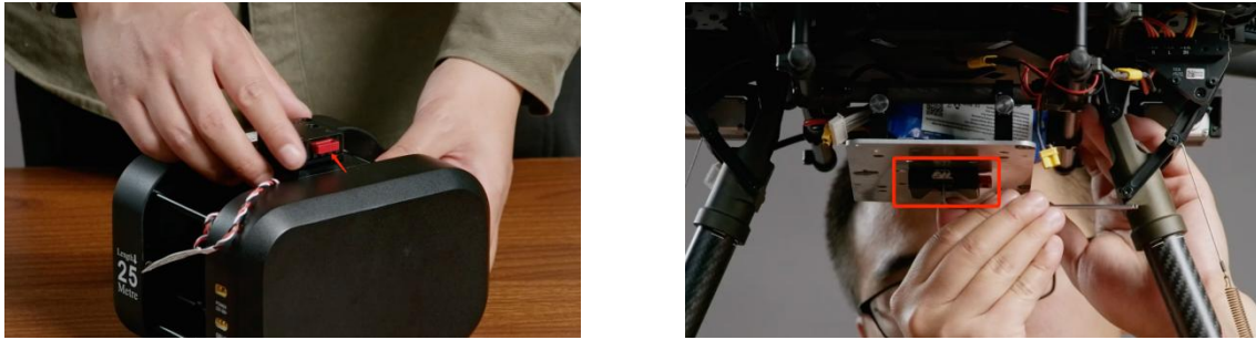
FIG 5-1-1 Show the quick-release mounting installation on drone
