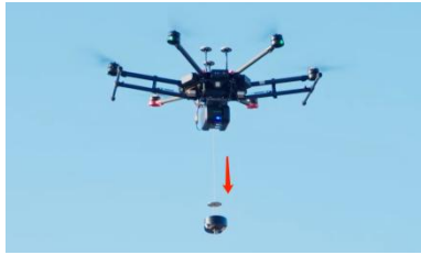
FIG 7-2-1 lower the rope to the ground
