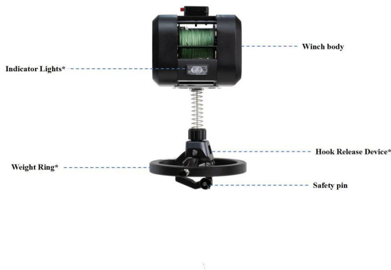
FIG 3-2-1 Diagram 1 of the XD-10 UAV payload winch
